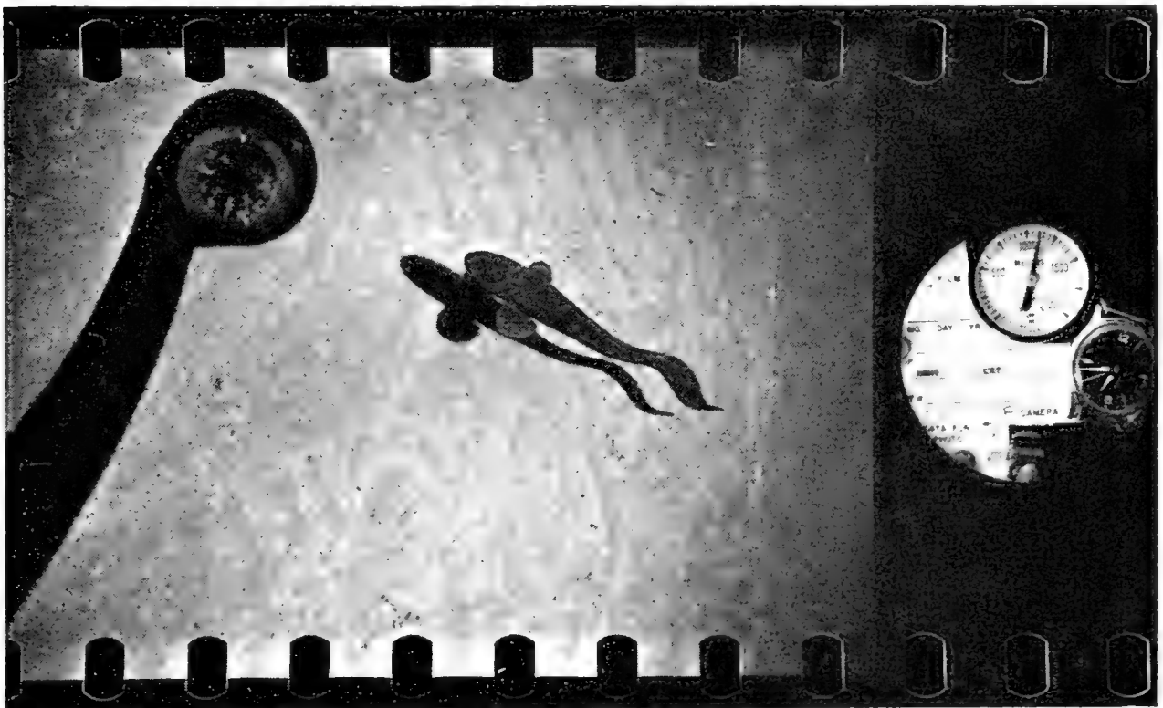
Fig. 5. One-half of a stereo pair of photographs taken from the R.V. Chain by the Woods Hole Oceanographic Institution at a depth of about 1100 m. The data section at the right shows pressure, time and other information. A compass in the field of view shows direction of the bottom.
